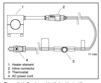
Figure 3-11 Crankcase Ventilation Heater Kit
